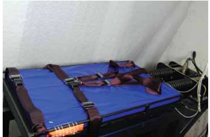
Figure 1: Test sled with stretcher and shoulder harness.
