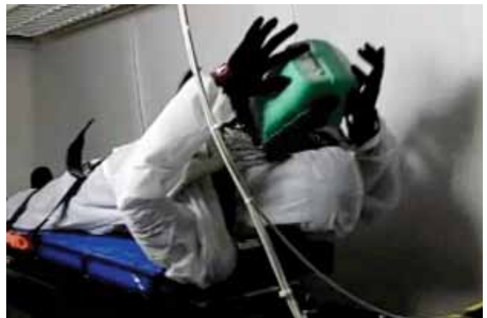
Figure 2: The top-heavy mass of the piston-driven system forcefully impacts the mannequin's head at 250 milliseconds.
