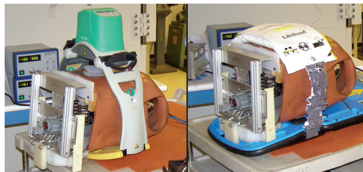
Figure 1: The piston-driven (left) and load-distributing band (right) systems shown applied to the calibrated mannequin.
